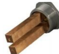
7" long 90% copper, 10% silver electrode, 3"sch 80 (CLE-20)
