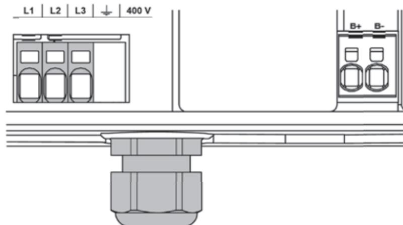
The connection terminals for the mains supply line are located inside the drive controller. Depending on the version, the assignment may differ. Wire end sleeves with plastic collar and flag are recommended.
