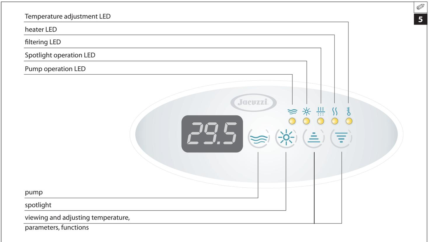
**NOTE ON THE “SILENCE” FUNCTION:** *where a timer or timer switch is installed, when activating the “Silence” function (see “Utility functions”) ensure that filtering is not scheduled during the time this function is active; in any case, the total filtering and “silence” time must not exceed 24 hours per day.*
